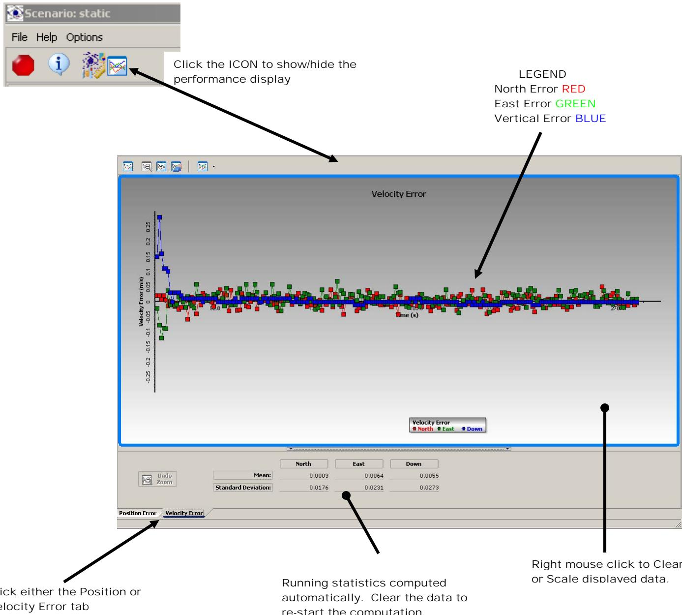
Note. The results displayed, the computed North, East, Vertical position and velocity errors, are saved in a file TEXT within the scenario folder. The file name is **POSVELERR.DAT**. You can import this file into Excel or an equivalent program. Also note, when you restart the simulation, the PosVelErr.dat file is overwritten so if you want to save it, copy it out of the folder before you restart the simulation.
